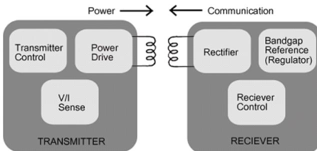
Figure 6.1: Basic block diagram of a four-part wireless power system
